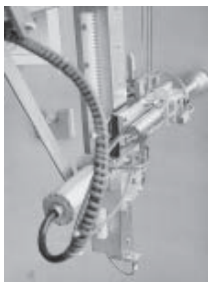
An area subject to radiation of up to 4 sievert/h whilst immersed in fully desalinated water in a manipulator for dismantling nuclear reactor pressure reservoirs and thermal shields.
