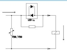
Each valve solenoid coil is protected with a spark arresting protective circuit as well as against polarity reversal.
