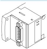
With this electrical connection variant, all valves are centrally actuated via the 15- and 26-pin connector plug.
