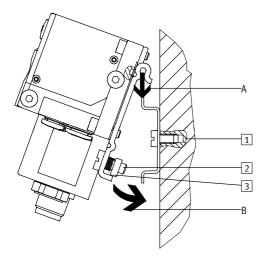
The CPVSC valve terminal is attached to the H-rail (see arrow A). It is then hinged on the H-rail and secured in place with the clamping component (see arrow B).
