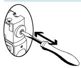
MO is actuated by pushing it with a pin or screwdriver and reset by spring force.
