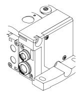
Exhaust from duct 3/5 as well as 82/84 via large surface area silencer Ducted exhaust air from duct 3/5 or 82/84
