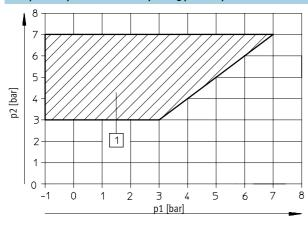
1 Operating range for valves with external auxiliary pilot air
