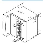
With this electrical connection variant, all valves are centrally actuated via the 20-pin connector plug. The electrical connection is located on the left-hand side.
