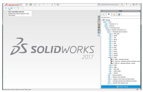
Festo's CAD plug-ins allow for a complete product selection process within the CAD system.
