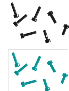
Fig. 121: Screws 1. Binarization, 2. detected as BLOB / object
