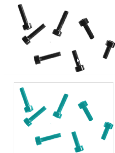
Fig. 121: Screws 1. Binarization, 2. detected as BLOB / object
