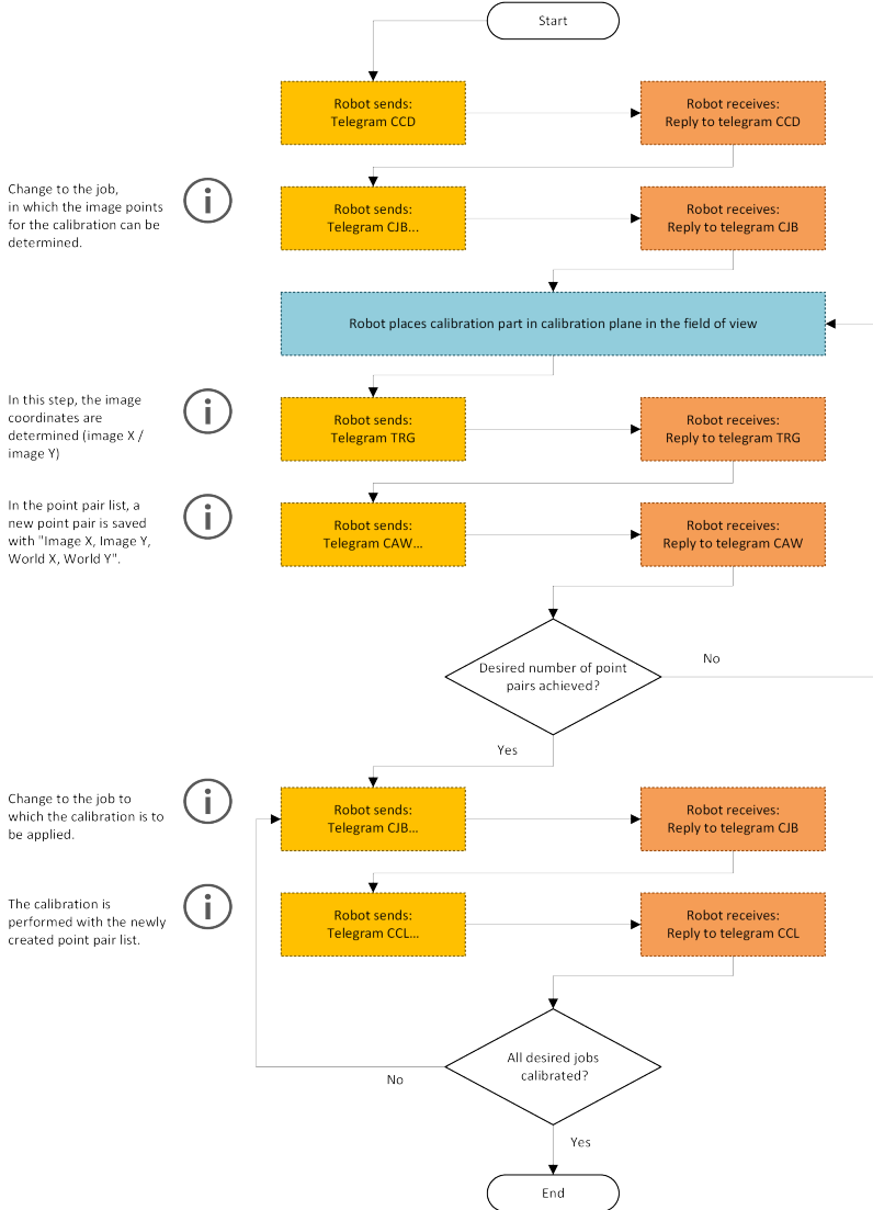
Fig. 60: Automated sequence for calibration via point pair list
