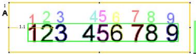
Fig. 148: Segmentation without any preset for parameter “Groups of characters”: All characters are found
