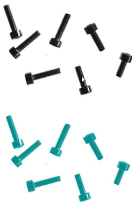
Fig. 1.16: Screws 1. Binarization, 2. detected as BLOB / object
