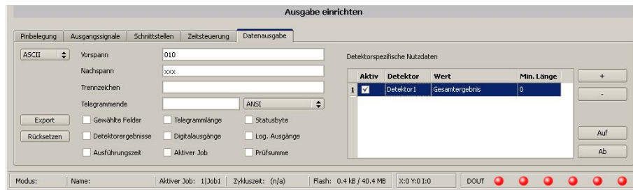
Fig. 235: Data output RS422, configuration of output data
