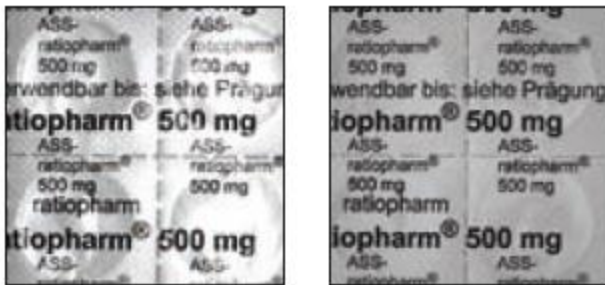
Fig. 223: left: spot illumination; right: diffuse illumination
