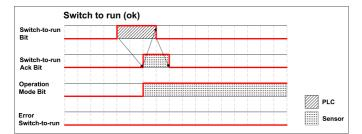
Fig. 25: Timing Switch to run ok
