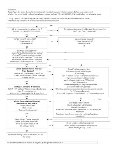
Fig. 2: Connection via network sensor / PC, procedure and troubleshooting
