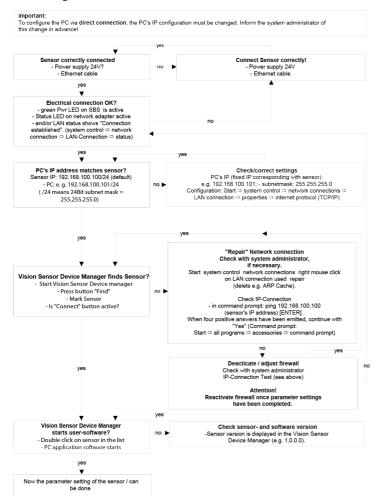
Fig. 1: Direct connection sensor / PC, procedure and troubleshooting
